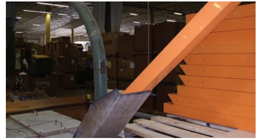
Recycling in the service of art: PVC gates from Christo's project "The Gates" being granulated.
