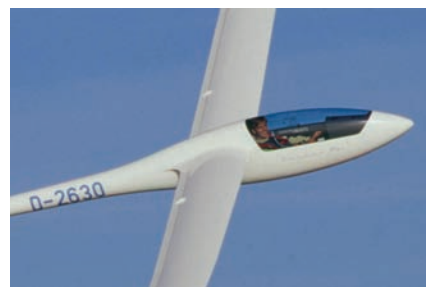
Light and stable: an aeroplane with sandwich construction and a foam core.
